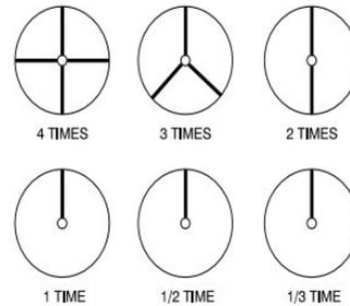
To measure true revolutions per minute (RPM) by Marking:
