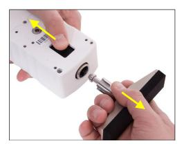
If the E1011 grip adapter (pictured below) is used, common grips and attachments may be mounted via the integrated 5/16-18F thread.
