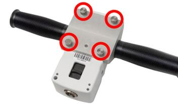
Attach the force gauge to the double handle grip (AC1003) or single handle grip (AC1003-1) by mating the male dowel pin in the cradle to the corresponding hole in the rear of the force gauge housing.
