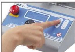
Measurement Start with the test stand start button.
