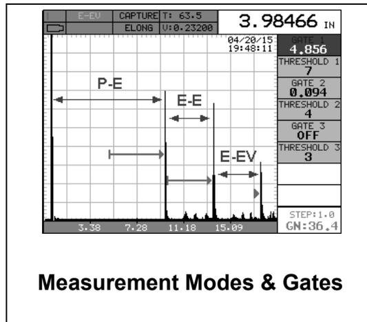
As stated above, the **MAX II** has a total of three gates depending on the measurement mode selected. The photo above illustrates the mode and number of gates needed for each measurement mode. One gate is used in pulse-echo, two gates for echo-echo, and 3 gates for echo-echo verify. The gates are fully independent, and starting positions and thresholds are the only adjustments available for each gate.
