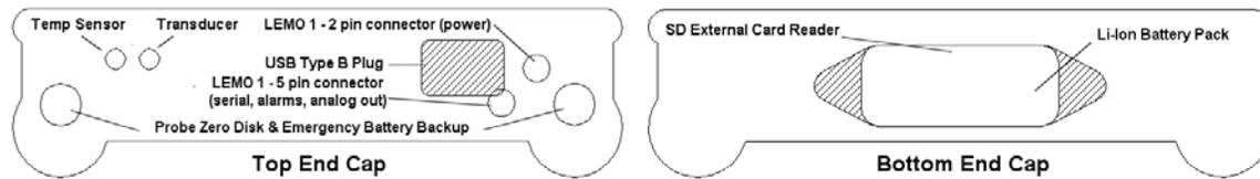
The top & bottom end panels are where all connections are made to the **MAX II**. The diagram above shows the layout and description of the connectors:
