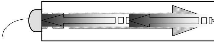
*Figure 1 Sound path in a good bolt*
