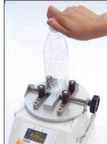
↑Opening PET bottle cap torque test
