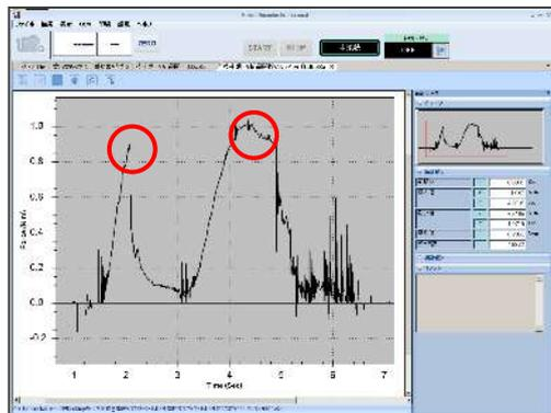
On the DTXA monitor, measuring 2 peak values and Max. value can be displayed at the same time.
