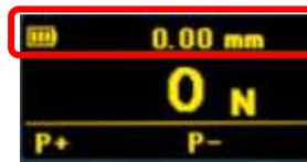
You can input/output displacement as well as force when you combine with a test stand having a linear scale by a dedicated cable or DMK scale. \*
