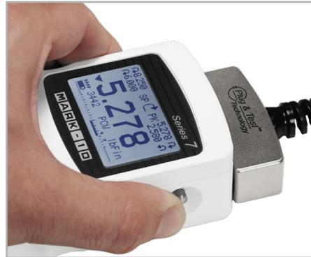
^ Unique Plug & Test® technology allows for interchangeable sensors to be used with a Mark-10 M71, M51 or M31 indicator. All calibration and configuration data is saved in the smart connector.
