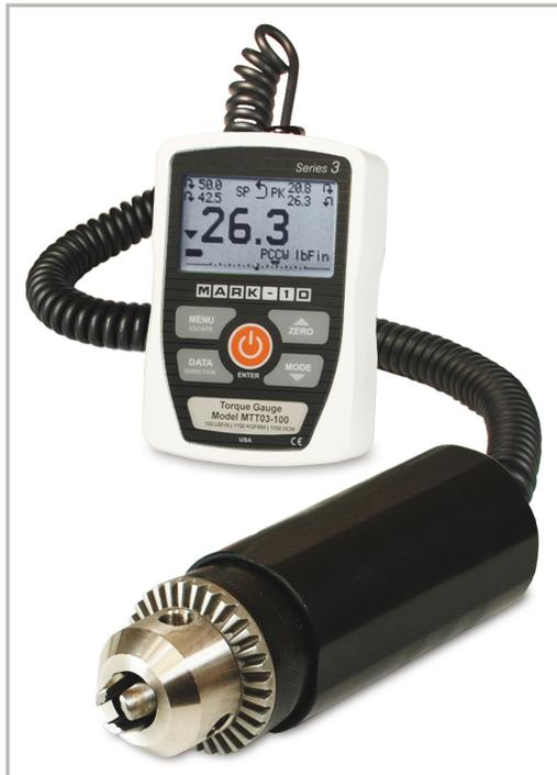
Series TT03 digital torque gauges are designed for clockwise and counter-clockwise torque applications in virtually every industry, with capacities from 10 ozFin to 100 lbFin (7 to 1,152 N). A dedicated remote torque sensor with Jacobs chuck can be used to grip a sample, bit, or screw. The gauges' rugged aluminum housing allows for hand-held use or test stand mounting to meet sophisticated testing requirements.
