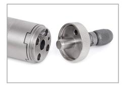
Series R51 feature unique interchangeability with three chuck attachment sizes as well as a bit holder. The attachment is mated to the main sensor body with a pin, while a threaded ring holds the attachment in place.
