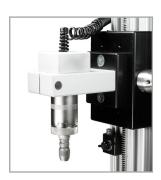
A Series R51 torque sensor is shown mounted to a model TSTM-DC motorized torque test stand using optional AC1015 mounting kit.
