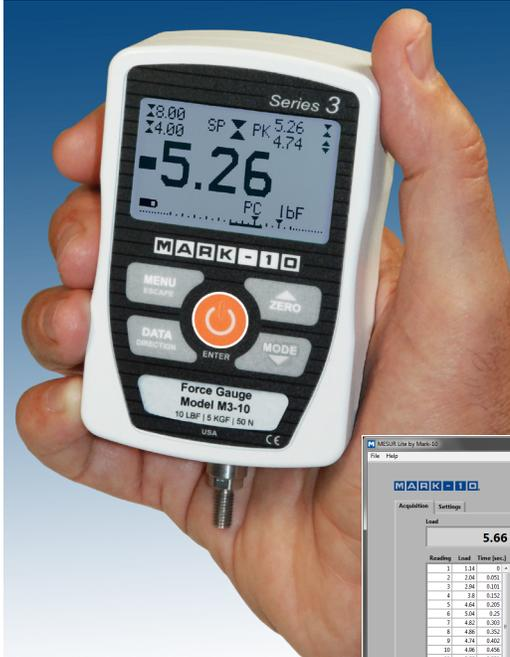
Series 3 digital force gauges are designed for tension and compression force testing in numerous applications from 0.12 lbF to 500 lbF (0.5 N to 2500 N). The gauges feature a sampling rate of 2,000 Hz, producing accurate results under a wide range of test conditions. A backlit graphic LCD displays large characters, and a menu is available to access the gauges' features and configurable parameters. USB output is provided for data collection purposes.
