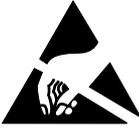
The MLT WESCO contains electronic components which can be destroyed by electrostatic discharge when touched. Therefore, all measures to avoid such discharge, e.g. by means of touching an earthed object (machine or earth contact of a plug, etc.), must be taken prior to opening the device.
