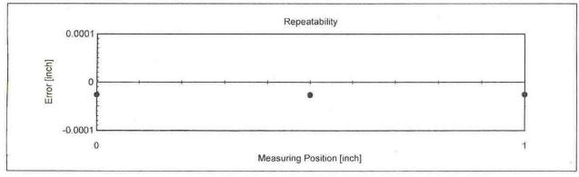
Repeatability is taken at three positions, with five readings at each position.
