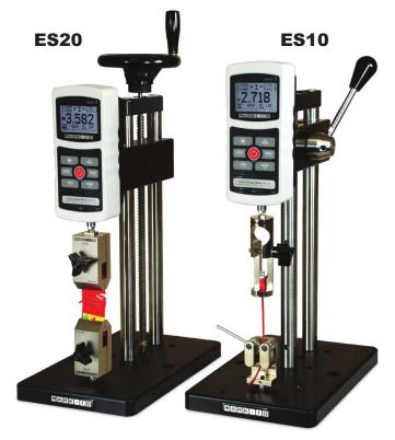
The ES20 is shown in a peel testing application with Series 5 digital force gauge, and film & paper grips.
